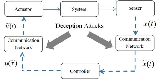
Fig. 1. Closed-loop framework of the system under attacks.
